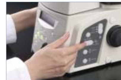
High-speed position changing of the filter cubes in 0.25 second
